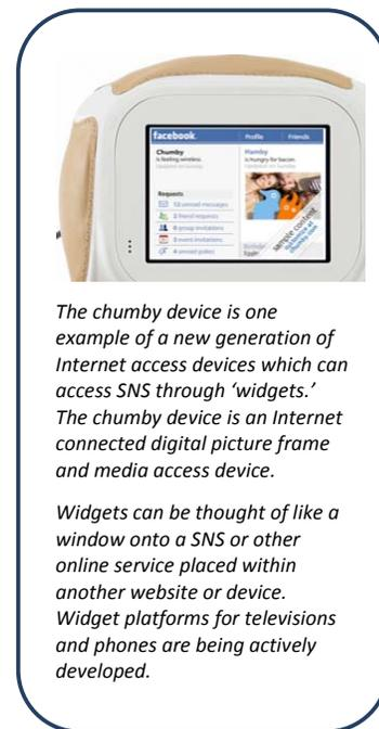
*The chumby device is one example of a new generation of Internet access devices which can access SNS through 'widgets.'*
